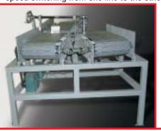
The switch consist in three conveyors mounted on a single rigid frame. One conveyor is pivoting around a vertical axis (from one side to the other), the two receiving conveyors are fixed.
